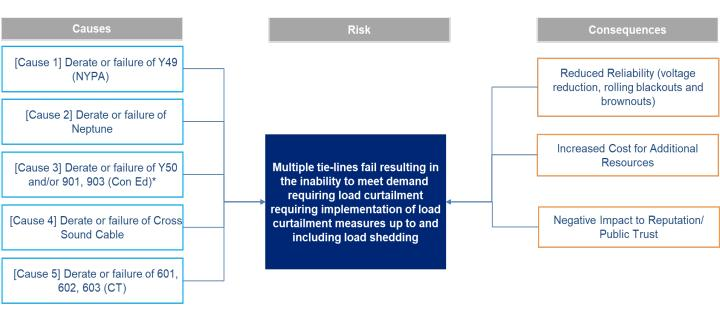
\*Note: 901 & 903 typically work in conjunction with the power imported on the Y50 intertie, and export power to Con-Ed
