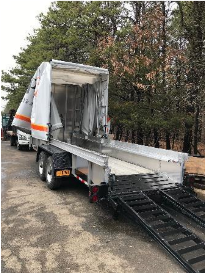
Trailer retrofitted with sliding load cover
