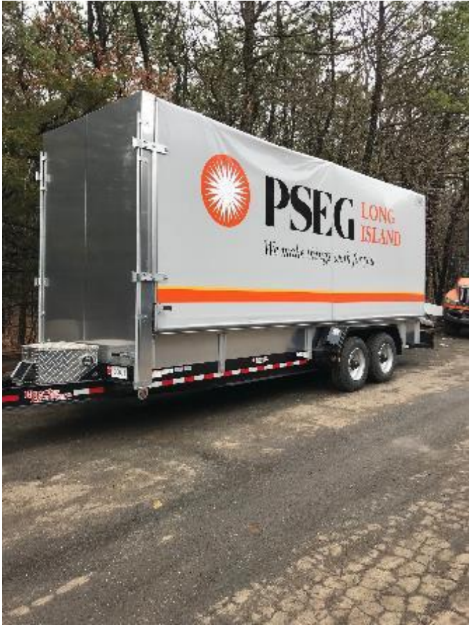
Trailer retrofitted with sliding load cover
