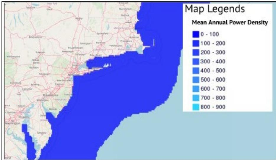
As noted from the data presented, the mean annual power density for tidal energy in the Long Island Sound is at the low end of the scale. Given the site's location in the Long Island Sound, there is little to no potential for the installation of a Tidal Energy system at the Northport station.
